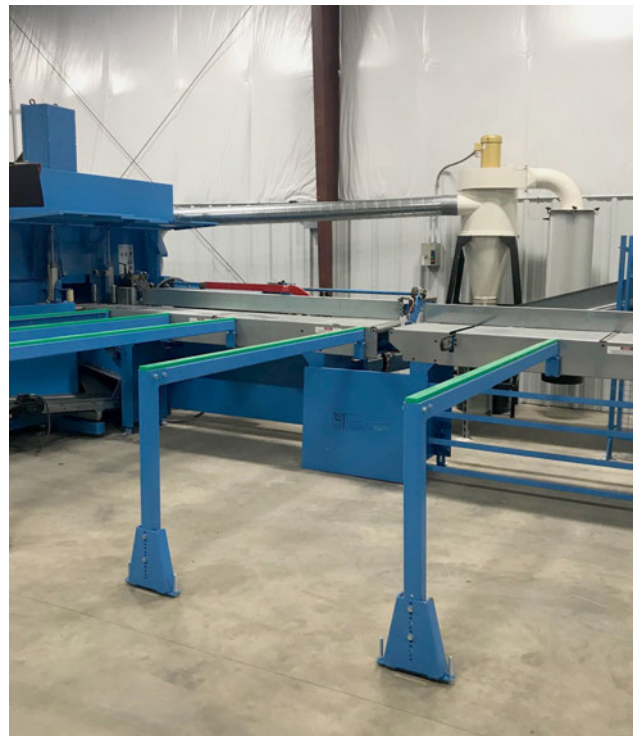
Oneida Air Systems' High Vacuum dust collector connected to a Hundegger CNC component saw.
